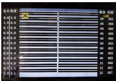
12 ribbon fiber accurate alignment
