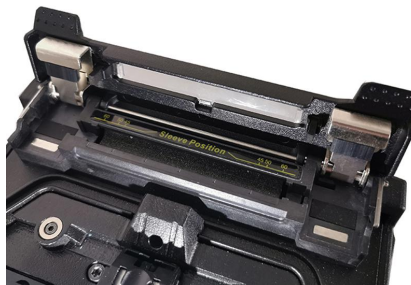
Inductive heater, without fiber not heating
